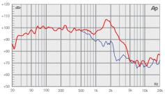
t Half space response measured in a 975 Litre sealed box.
